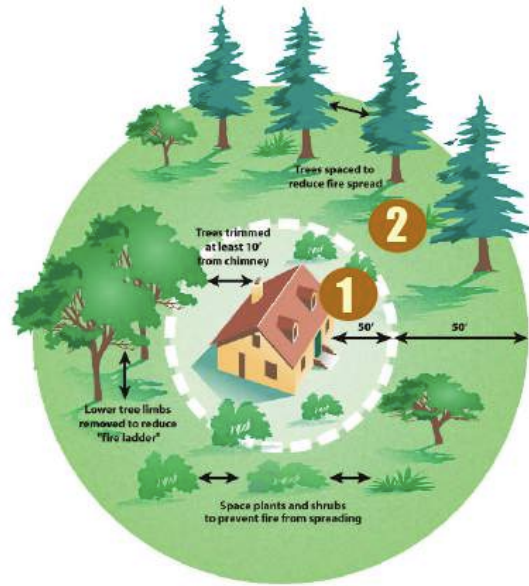
Figure 4. Defensible space zones around structures. 28
