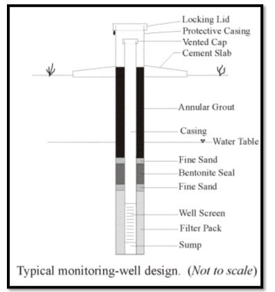
Figure 81. Depiction of a typical Piezometer Installation
